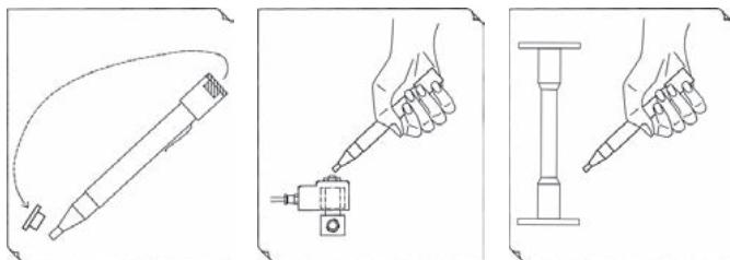
MasterEx 79784 is a pen-sized magnet probe, designed to detect magnetic fields in hazardous areas. Within seconds it is possible to detect whether or not a solenoid valve is electrically activated.
